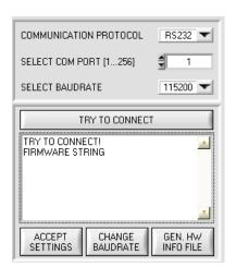
The baudrate for data transfer through the RS232 interface can be set by means of the **SELECT BAUDRATE** drop down menu and **CHANGE BAUDRATE** function field.
