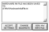
A click on the **GEN. HW INFO FILE** generates a file in which all the important sensor data are stored in encrypted form.
