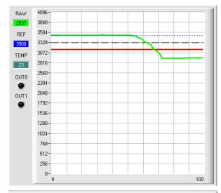
When the current measurement value **RAW** (green line) falls below the switching threshold (red line), the output **OUT0** changes to OV (error). This is visualised by the **OUT0** LED.
