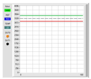
As long as the current measurement value **RAW** (green line) lies above the switching threshold (red line), the output **OUT0** has +24V (signal is OK). This is visualised by the **OUT0** LED.
