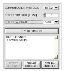
Now a new baudrate can be selected under **SELECT BAUDRATE**. A click on **CHANGE BAUDRATE** sends the new baudrate information to the sensor.
