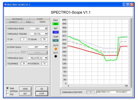
In this example a value of 50 was specified for **TT DOWN**. This means that downward threshold tracing is performed at a relatively slow speed.
