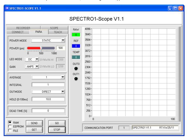
The window size and position will be the same as when the software was last closed. A double-click with the right mouse button e.g. under the minimise symbol places the window centrally in its original size.
